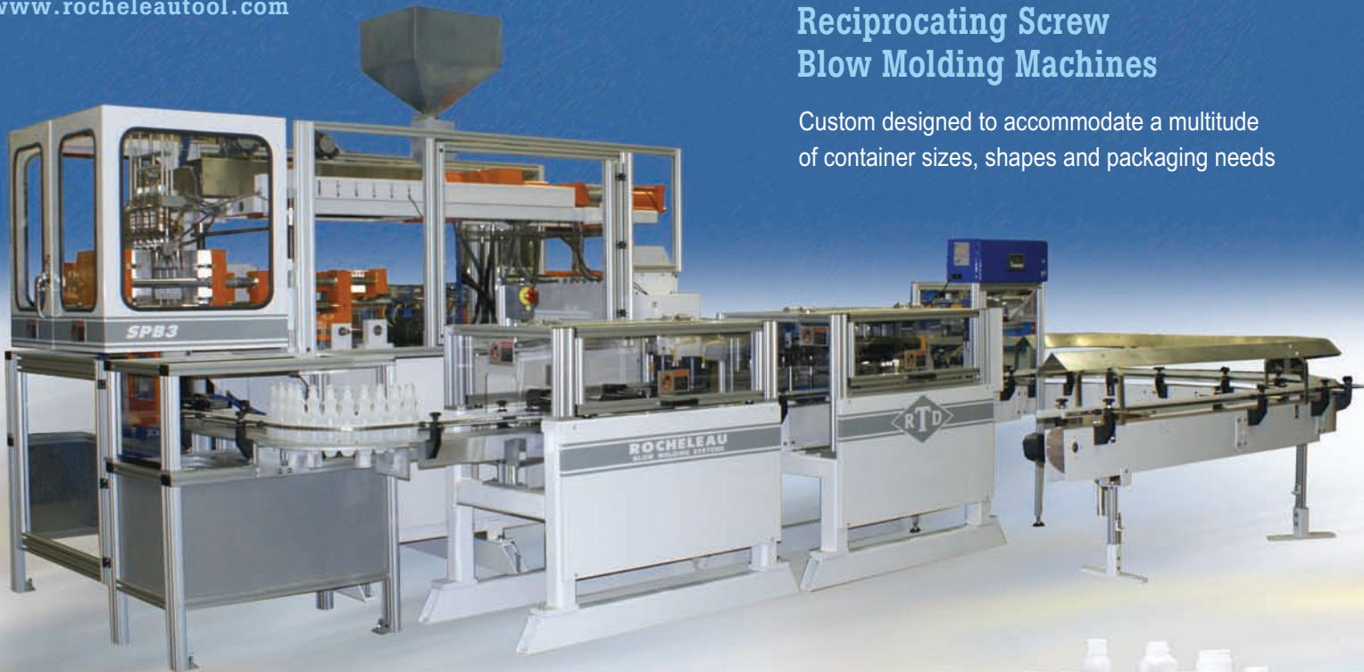
SPB-3 with SPB/HT1 Tail Puller and Spin Trim Take Away, In-Line Leak Testing
